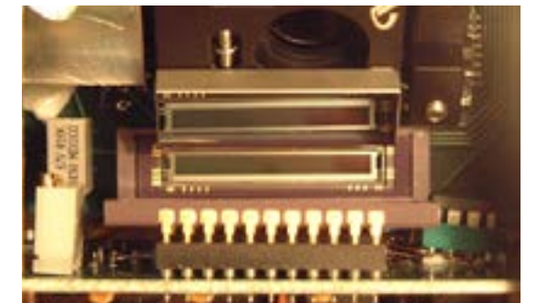
Diode array detection head for a small spectrograph.
